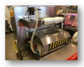
This Unimec Slypack Evo tray sealer has a vacuum/ gas setup and currently runs a 11x9 tray mould
